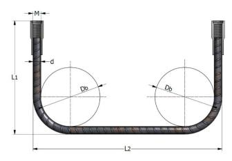
Other lengths are available on request  $PSAGGD - d \; x \; L_1 \; x \; L_2 \text{in mm}$
